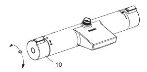
Rotate control handle(10) in clockwise/anti-clockwise 90° to transfer functions (Spout/off/handheld shower/shower head)
